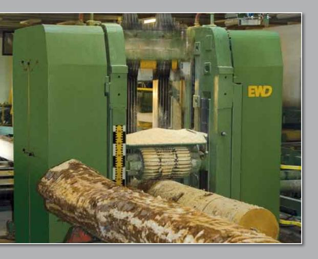
Heavy-duty sash gang saw for the use in medium to large sawmills
