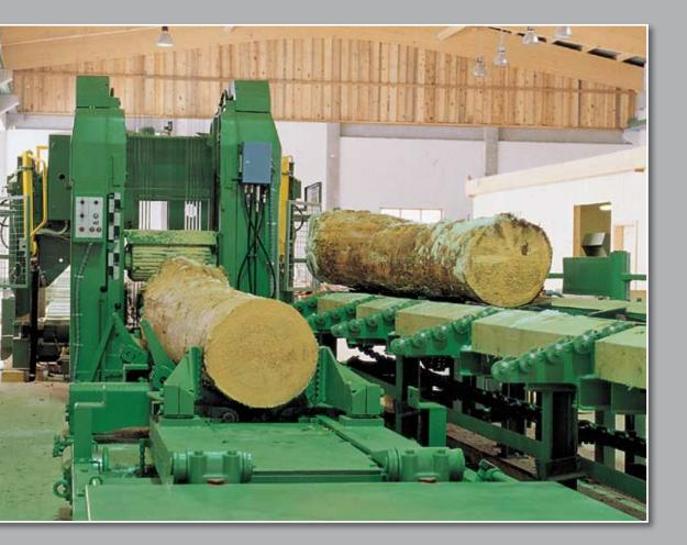
Heavy-duty oscillating frame sash gang for best surface qualities and high feed speed
