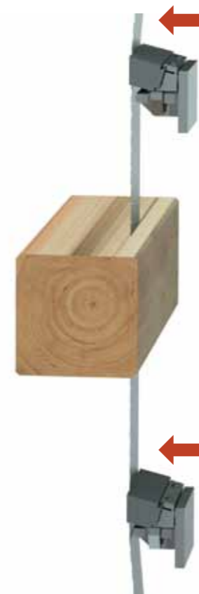
Passage of the band through the lumber with pressure guides
