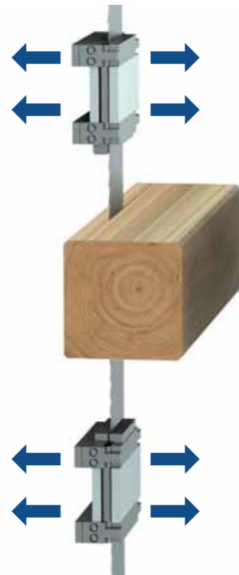
Passage of the band through the lumber with active magnet guides (FBS-Technology)
